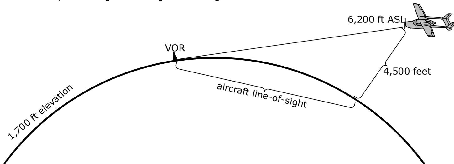
$$\begin{aligned} \text{Aircraft\_height\_above\_VOR} &= \text{aircraft\_altitude\_ASL} - \text{VOR\_elevation} \\ &= 6,200 \text{ ft} - 1,700 \text{ ft} \\ &= 4,500 \text{ ft} \end{aligned}$$
