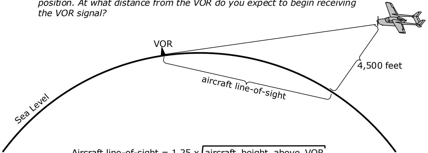
$$\begin{aligned} \text{Aircraft line-of-sight} &= 1.25 \times \sqrt{\text{aircraft\_height\_above\_VOR}} \\ &= 1.25 \times \sqrt{4,500 \text{ ft}} \\ &= 83.9 \text{ nm} \end{aligned}$$
