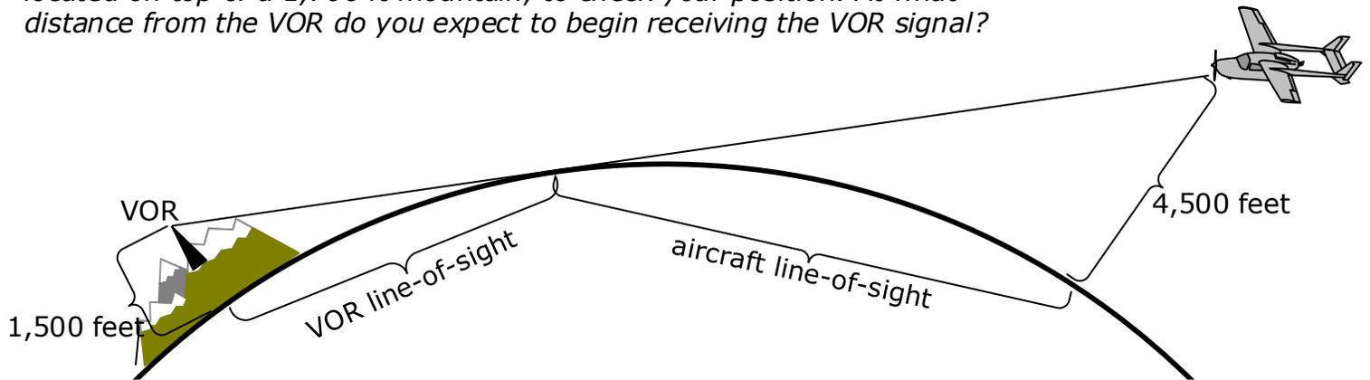
The VOR operates on VHF frequencies, whose maximum reception range is line-of-sight. However, if the radio waves just skim over the surface of the earth then they continue to propagate as shown in the diagram above.
